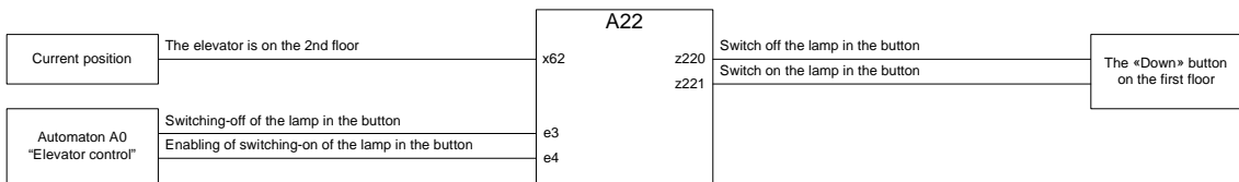
Fig. 12. A link diagram for the "Down" button of the second floor" automaton
